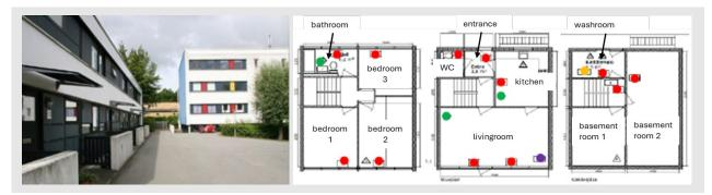
Figure 4 Picture of the case study building (left). Location of the radiators (red circle), temperature sensor (green circle), fireplace (purple circle), and DH substation (yellow) (right). [34-41]
