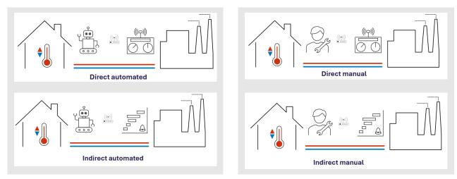
Figure 3. Illustration of the four types of DR according to Annex 84
